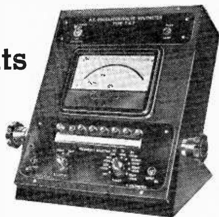
Fig. 1. Combined a.f. oscillator and output meter for routine testing of amplifiers and tape recorders.
